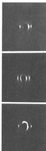
FIGURE 1 X-ray diffraction photographs of 9 OBCAB in (a) smectic A phase at 140^\circ\text{C} , (b) reentrant nematic phase at 100^\circ\text{C} , and, (c) reentrant smectic A phase at 68^\circ\text{C} .
